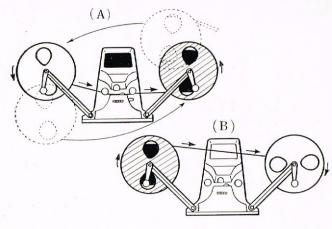
(9) For fast rewinding, place the take-up reel on the left arm as per figure (B).
