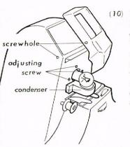
(10) To change the projection lamp, unscrew both sides of the screen cover.
